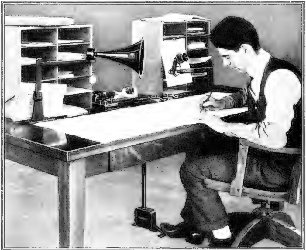
The apparatus reproduces the exact tones of the speaker's voice but with magnified volume and clearness, so that a whisper would be distinctly audible under ordinary conditions
